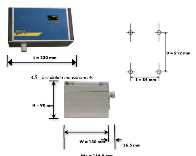
W+=156.5 mmOpen/close the gas detection control unit, remove it from/install it via the back panel by screwing in/unscrewing the housing screws (M3 flat screwdriver or M3 Phillips head screwdriver).
