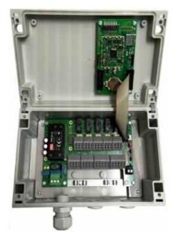
Upper part with CPU board, display for operation and visualization of measured values 3 adjustment buttons (keypad) Connection pin socket (P3), for connecting cable and USB cable, DIP switch and a button battery
