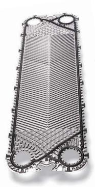
*Gemini:* With their double walls, our Gemini plates combine excellent heat transfer with increased protection against the mixing of fluids. The plates consist of two sheets that are formed together, which prevent the media from mixing, even in the event of a cracked plate. Gemini plates are available on both Alfa Laval FrontLine and BaseLine models.
