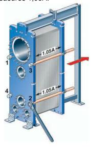
Step 2: Loosen the two diagonal pairs of bolts are loosened alternately, as shown in the figure below.
