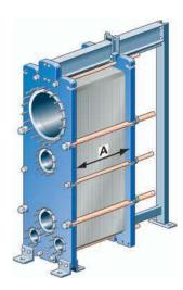
Loosen the bolts which are not fitted with bearing boxes and remove them.
