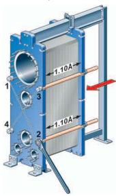
Step 2: After that bolts are tightened alternately and diagonally, as shown in the figure below. Check the dimension A during tightening at the positions of the bolts that are being used.
