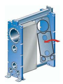
Press the plate assembly together. Tightening is done in two steps, see figures below. Be careful so that the frame plate and the pressure plate are always in parallel.
