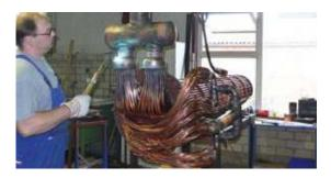
Two 6,500 litre tanks connected in paralell with each having four single circuit evaporator, and four independent refrigeration systems for Doha airport. This application is for brine cooling -8/-3°C:
