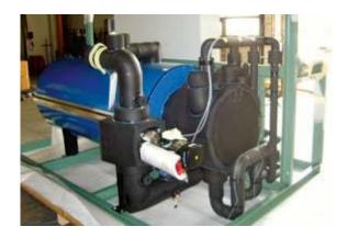
llustration of tank and evaporator for cooling mediums -40°C being prepared for international engine test standards for international automakers.
