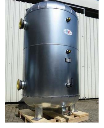
The larger and special dimension tanks are normally supplied without fitted insulation and must be insulated on site after installation and assembly. All tanks can also supplied with insulation (made of vinyl rubber with and without metal jacket). DK has in planning a suitable insulation for outdoor installation (with rear ventilation).
