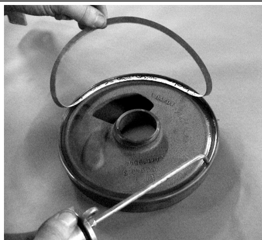
12. Lightly oil the grooves of the intermediate rings.
