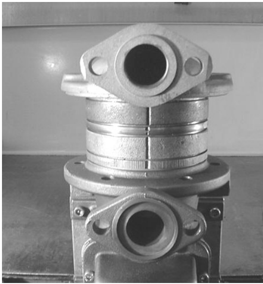
15. Assemble the intermediate rings and gaskets (33) in such a way that the marks align.
