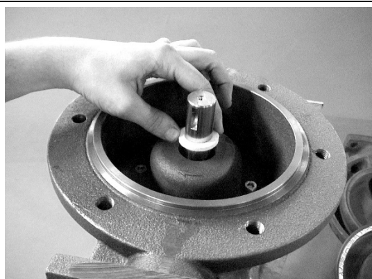
9. Inner Sealing: Use the same procedure as described in the two photos before.
