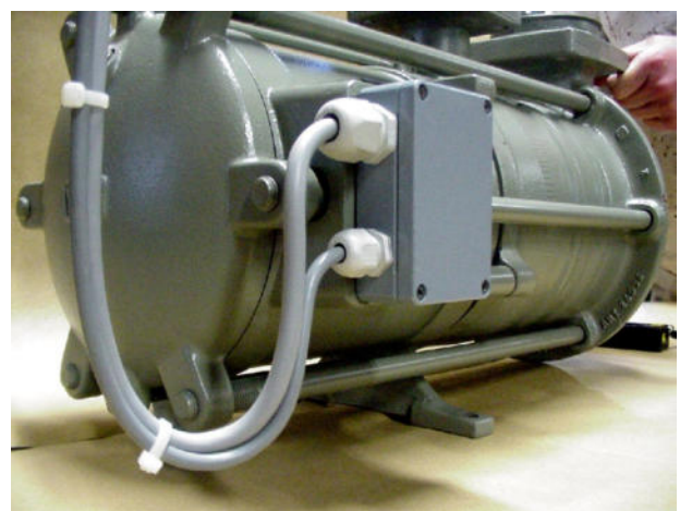
Fig.9 b Correct connection with loop in electrical cable
